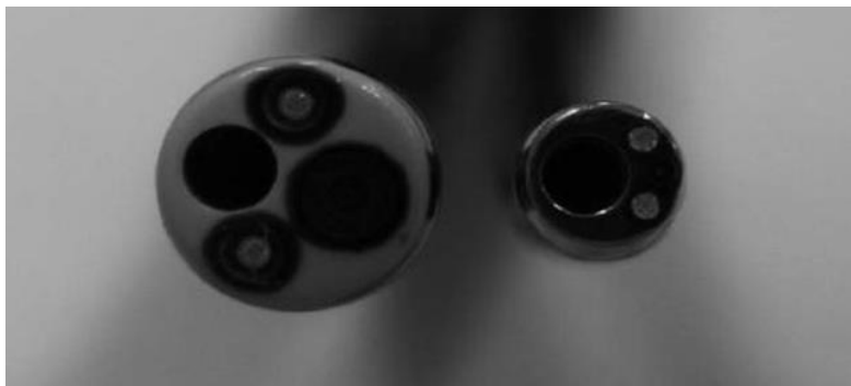
Figure 6. Standard bronchoscope with a distal end diameter of 5.9 mm and a working channel of 2.0 mm (BF-240; Olympus, Tokyo, Japan). b) Thin bronchoscope with a distal end diameter of 3.5 mm and a working channel of 1.7 mm (XBF-3B40Y1; Olympus). Oki M et al. Novel thin bronchoscope with a 1.7-mm working channel for peripheral pulmonary lesions. European Respiratory Journal 2008 32: 465-471.
