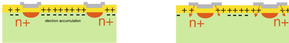
Figure 3.7 Strips implant and readout design. Non-sharp edges (left) and enlarged profiles are desired. Wider Aluminium readout (right) can be used to avoid high fields and electron accumulation close to the implants.
