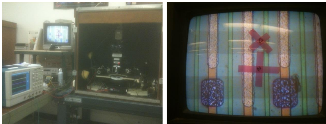
Figure 6.88 Laser injection system and measurement equipment (left). Detail of the alignment precision (right). The marks correspond to two different lenses. For this work the “+” mark is used as reference.
