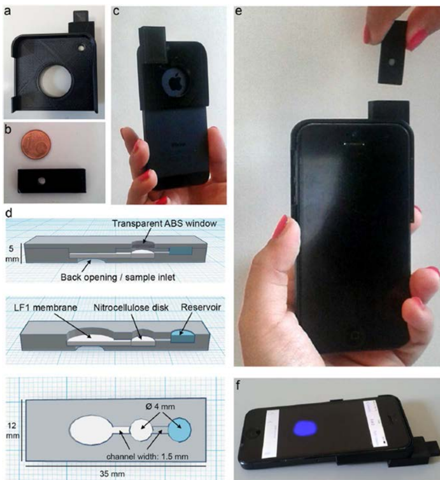
Fig. 8. Adapter for chemiluminescent strips reading. (a), (b), (c) images of the devices, (d) scheme of the cassette for the strips, (e) coupling of the cassette on the mobile phone and (f) signal procurement. Adapted with permission from Roda et al. (2014b) . Copyright 2014 American Society of Chemistry.
