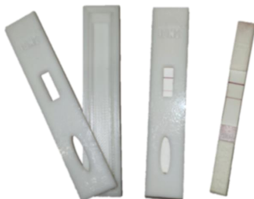
Fig. 0.1. Lateral flow device. From left to right: 3D-printed cassette, lateral flow strip in a 3D-printed cassette and a single lateral flow strip.
