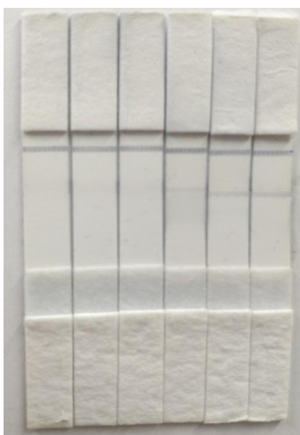
Fig. 0.3. Iridium oxide (IV) nanoparticles-based lateral flow strips, first time reported in this thesis work.
