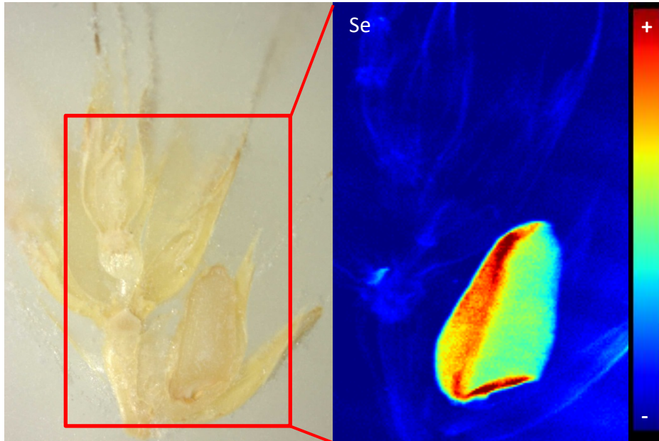
Figure 14: Study of the selenium distribution in a section of the ear of a senescent plant, containing one grain. Visible image obtained by a microscope, with the area studied by XRF marked by a red square. Selenium fluorescence map, where higher concentrations are shown in warmer colors and lower concentrated regions appear in blue, as indicated in the legend.
