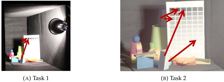
FIGURE 2.4: In Experiment 1, observers performed two tasks. In Task 1 (A), observers had to match the brightnesses of the 5 cuboids' facets to the brightnesses of 5 patches in the reference table. In Task 2 (B), observers had to perform the same task on the TMO image displayed on the calibrated monitor. Red arrows are randomly drawn just for illustrative purposes.
