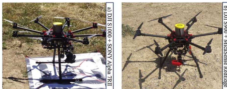
Fig. 4. a) Octocopter platform with the RGB sensor mounted on the gimbal; b) Hexacopter platform with the multispectral sensor mounted on the gimbal.
