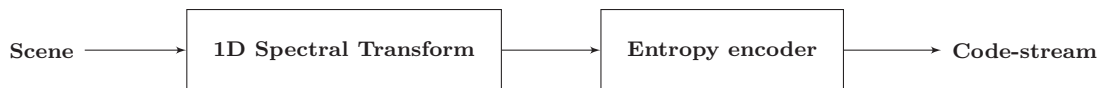
Figure 6.1: Pipeline of our coding systems: 1D spectral transform followed by JPEG 2000 or CCSDS-123-AC.
