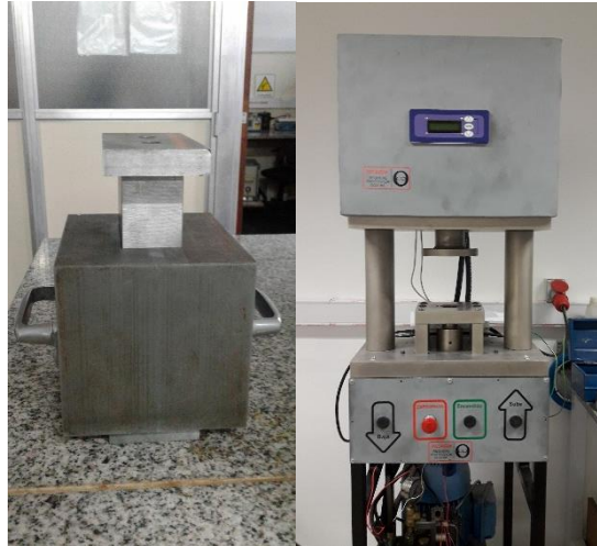
Figure 3.43 Mold and press machine used to make bricks.
