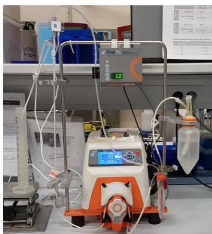
Figure 13. Image of the diafiltration system for QS purification.
