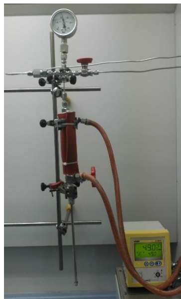
Figure 10. Schematic representation of the lab-scale set-up (left) and image of the reactor (right) used for the DELOS-SUSP experiments.
