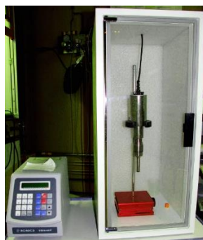
Figure 12. Image of the Vibracell Sonicator used for nanostructures preparation.
