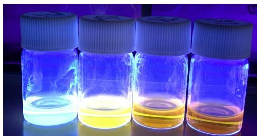
Figure 33. QRs produced using meta -carboranephosphinic acid as capping agent. These images show QRs pipetted out at 45s, 1 min, 5 min and 15 min respectively (from left to right) after Se addition. These images were taken under UV illumination at a wavelength of 365 nm.
