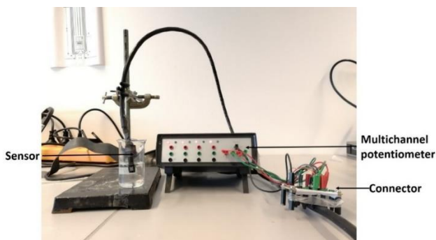
Figure 10. c) A single-device electrochemical cell operating simultaneously with four WEs enabling to perform electrochemical measurements in small volumes.
