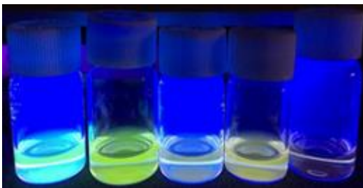
Figure 4. QDs produced using meta - carboranethiol as capping agent. These images show QDs pipetted out at 20s, 30s, 45s, 1 min and 5 min
