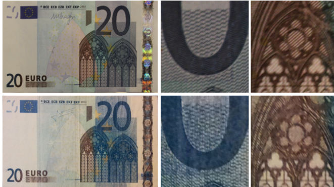
Figure 1.1 – Example of resolution loose in fine-line patterns. First row €20 genuine banknote and ROIs extracted, second row scanned and printed €20 counterfeit banknote. Acquired with BQ Aquaris M5 smartphone at 600 dpi.
