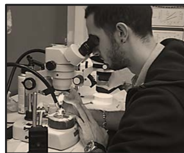
Figure 2.1 The author of the present work, using magnification lenses to manually introduce a fragment of a sample (of only a few tens of micrometers in size), inside the 0.25 mm diameter hole of a metal gasket, used for pressure generation.
