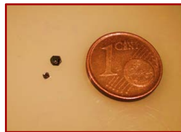
Figure 2.2 Example of two of the \text{MAPbI}_3 single crystals used in this thesis, grown at Bath University. A 1 cent coin is placed next to them for perspective.
