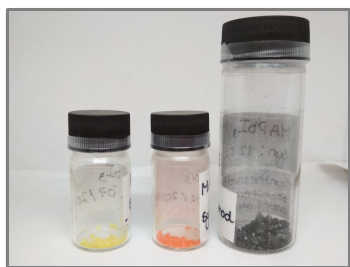
Figure 1.2 Example of perovskite crystals used during this thesis. From left to right: \delta -phase of \text{FAPbI}_3 , \text{MAPbBr}_3 , and \text{MAPbI}_3 crystals synthesized by our colleagues in Bath.
