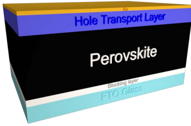
Figure 1.5 Example of a p-i-n heterojunction architecture for a fully perovskite solar cell.
