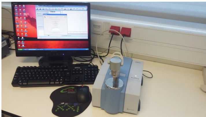
Figure 3.35. The ATR-FTIR equipment used, in this study, for the quantitative analysis of nanocomposites.
