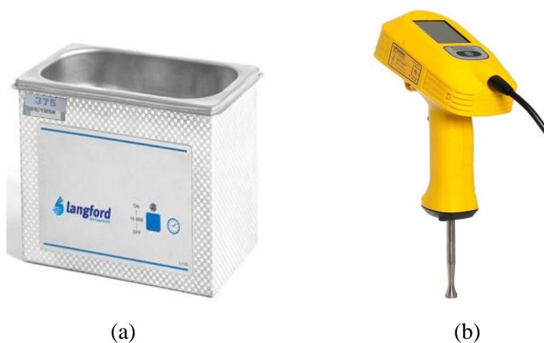
Figure 3.22. (a) Ultrasonic bath and (b) ultrasonic probe used in the current study to disperse MWCNTs.
