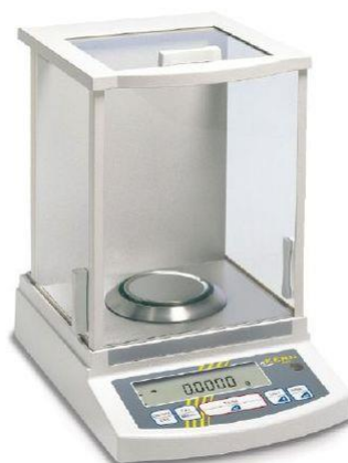
Figure 3.18. The electronic balance used in the current study to prepare different compositions.
