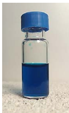
FIGURE 2.9: Image of a YBCO precursor solution with a 12% molar \text{LaF}_3 nanoparticles content.
