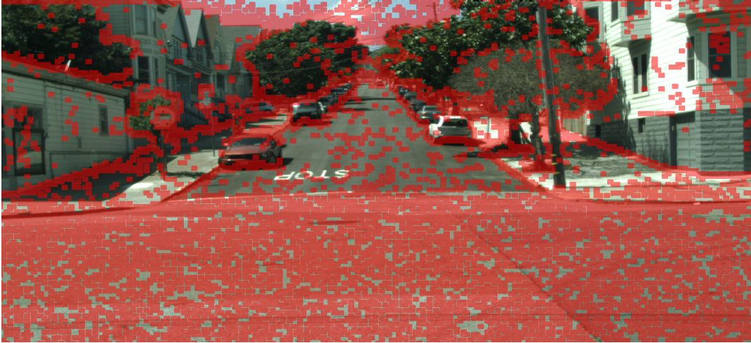
FIGURE 3.6: Generated Stixel cuts (highlighted in red) using the left and right extrema as defined in [31], and also cuts generated from semantic segmentation. Stixel cut density is 30%, equivalent to a 3.3\times reduction in vertical resolution.
