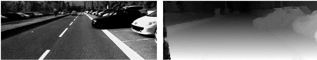
(A) Image obtained from the left camera of the car (B) Disparity computed with SGM described here
