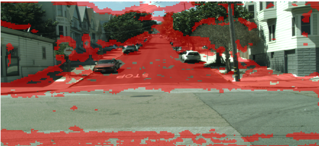
FIGURE 3.7: Generated Stixel cuts (highlighted in red) for the FCN-based method. Stixel cut density is 31.5%, equivalent to a 3.2\times reduction in vertical resolution.
