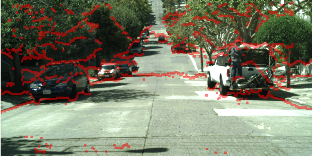
FIGURE 3.9: Sample image from the real-data sequence used for Stixel cut generation. Stixel cut ground-truth is highlighted in red.
