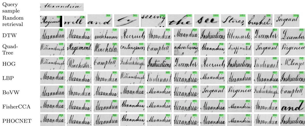
Figure 3.8: Qualitative example of retrieval results of the methods for a randomly selected query (Alexandria). From left to right: the nearest samples retrieved by each method. The id of each sample which distinguishes different samples with the same text is marked in superscript (green). Best viewed in pdf.
