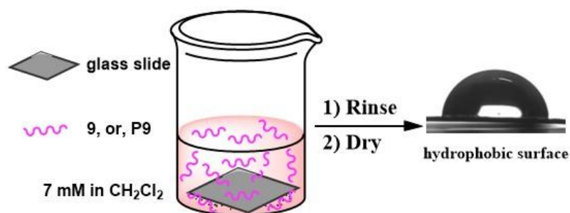
Figure 4.14. Schematic representation of coating procedure. The glass slide is submerged into the solution for at least 4 h, washed and dried before measuring WCAs.
