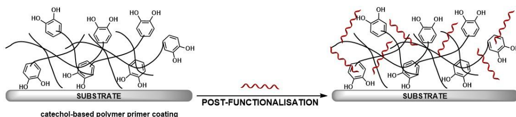
Figure 4.2. Illustration of the functionalisation of a primer catechol-based polymeric coating with a hydrophobe.
