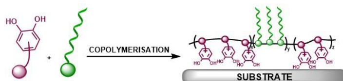
Figure 3.7. Polymerisation of molecules containing catechol moieties and PEG chains through reactive pendant groups. Coatings via ex situ treatments.
