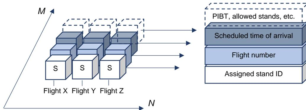
Figure 6. Stand assignment schedule coded for a genetic algorithm in Module II
