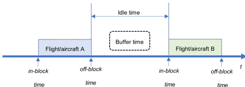
Figure 3. Illustration of idle and buffer times in the gate/stand assignment plan
