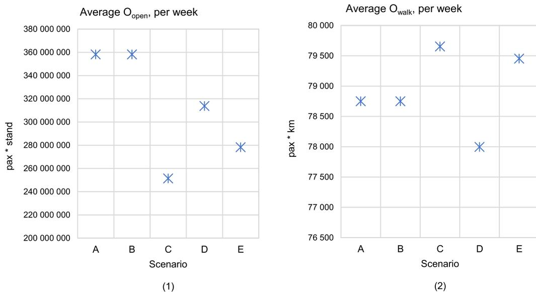
Fig. 5. Experimental results for the passenger-weighted number of aircraft assigned to remote stands  $O_{open}$  (1) and transfer passenger-weighted walking distance  $O_{walk}$  (2).
