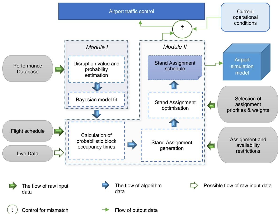
Figure 4. DASA framework architecture and primary data flows
