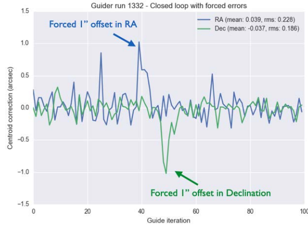
Figure 2.14: A guiding test in ProtoDESI where we manually moved the telescope tracking by 1" and the guider picked up the jump and recovered back to its center to continue the guiding process.
