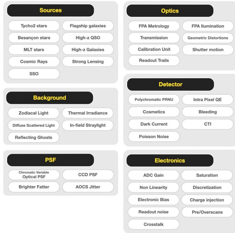
Figure 4.15: A summary of all the sources and instrumental effects in the VIS simulator.
