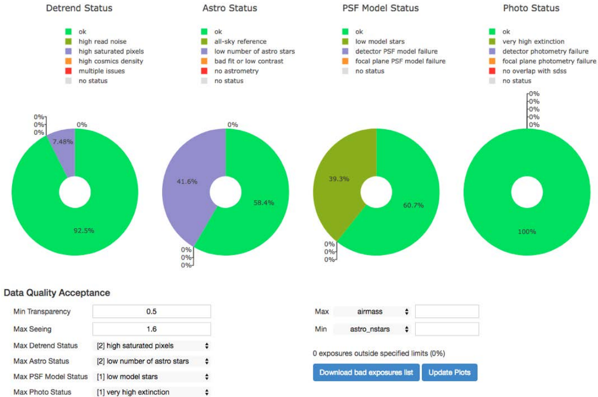
Figure 3.52: The selection tool from the nightly report showing the status of the main 4 sections in the nightly pipeline. It allows to set limits specified by the survey to re-observe the targets that did not meet specific quality requirements.
