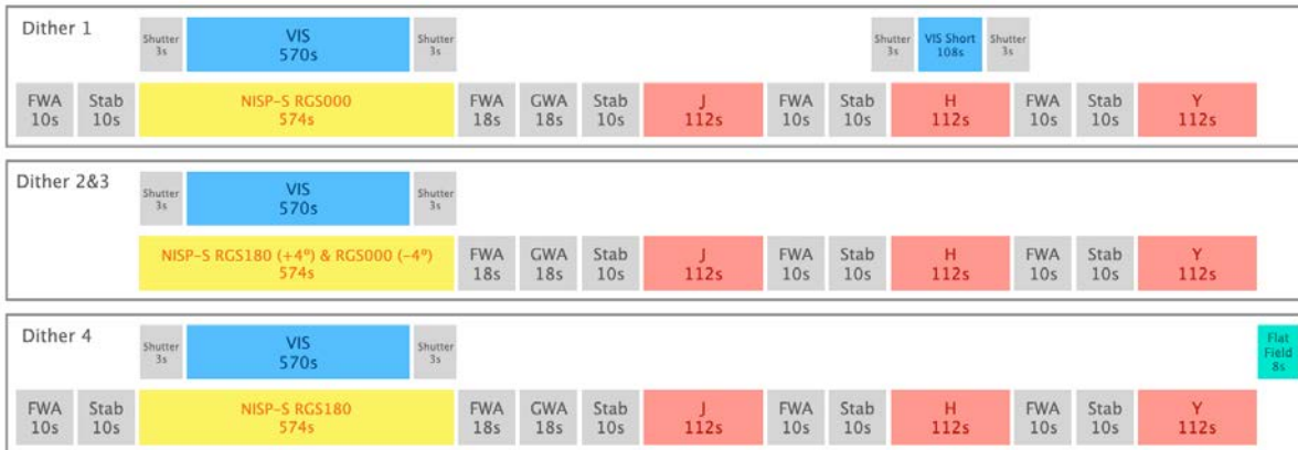
Figure 4.13: The reference observing sequence (ROS) in the four dithers for the VIS and NISP channels. At the beginning of each dither VIS and NISP-S observe simultaneously after the Filter Wheel Assembly (FWA) and few seconds to allow the telescope to stabilize. After the exposure, the Grism Wheel Assembly (GWA) lets the light pass for the filter observations of J, H and Y. The first dithers includes an additional short VIS exposure while the last dither ends with a brief flat field frame.
