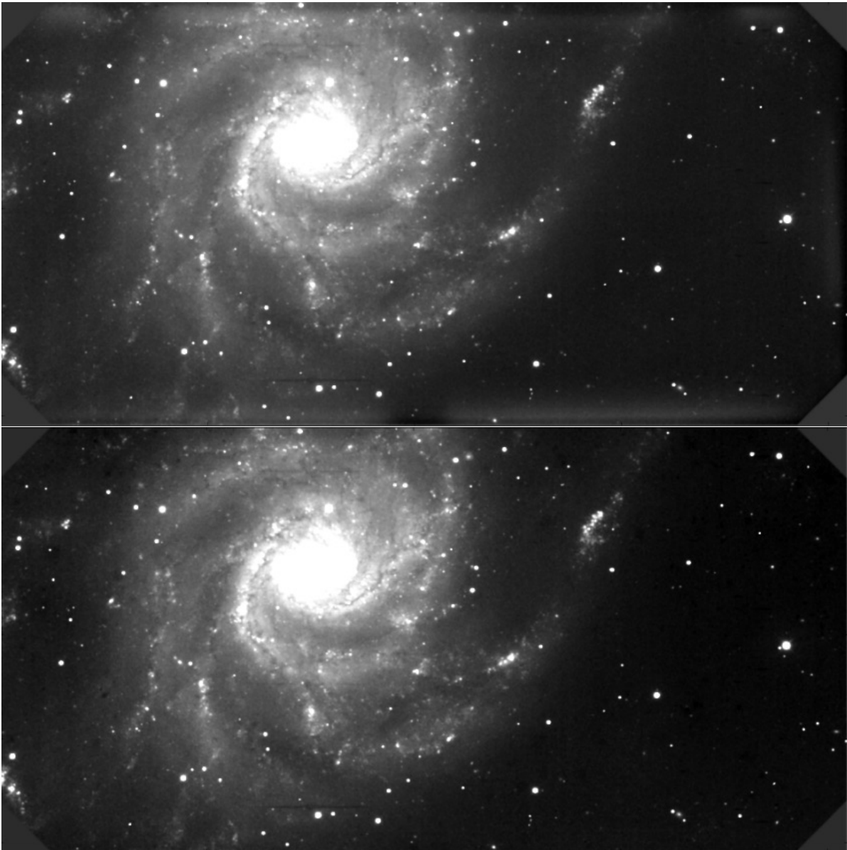
Figure 3.32: This figure shows how sky flats can correct for scatterlight and preserve light from extended sources (M101 in the pictured image).
