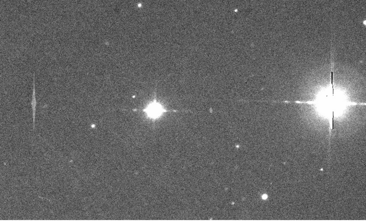
Figure 3.26: On the right of this crop image an 8.5 magnitude star saturates the detector producing bleeding and a visible crosstalk signal on the mirrored amplifier in the left side of this image.
