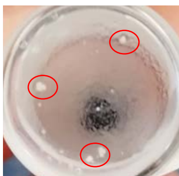
Figure 50. Non-reconstitutable precipitates were produced in batch 21 marked with red circles.
