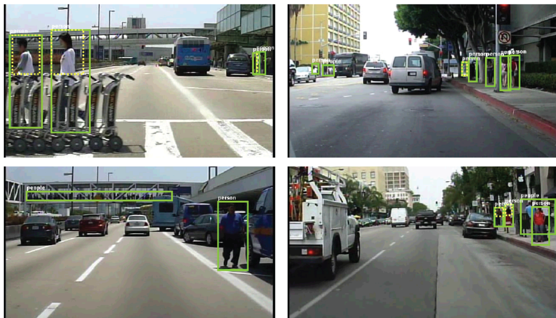
Fig. 3.1 Example images from Caltech Dataset with annotations [99]. Pedestrians can be detected as a single person or as a group of people. The solid green boxes indicate full person or people detected. The yellow dashed boxes indicate the visible part of a pedestrian detected.
