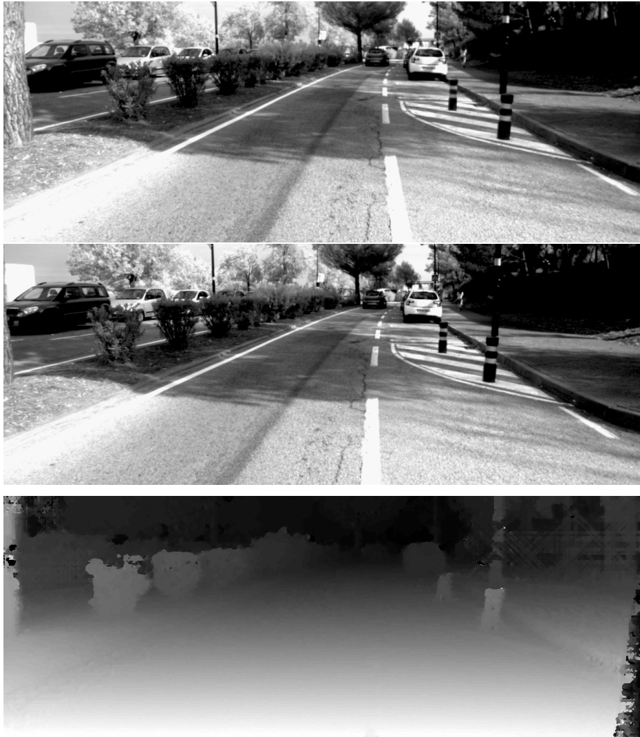
Fig. 2.7 Example of the disparity map computed using SGM from stereo images provided in [23]
