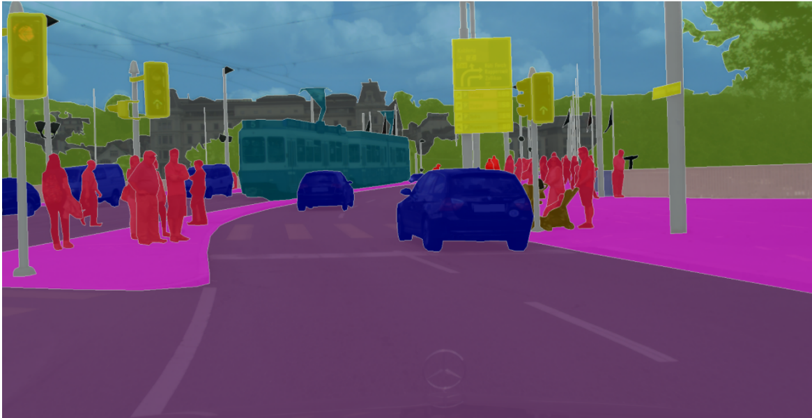
Fig. 2.8 Semantic segmentation example Cityscapes dataset [26]. Objects in the same class have the same annotation color.
