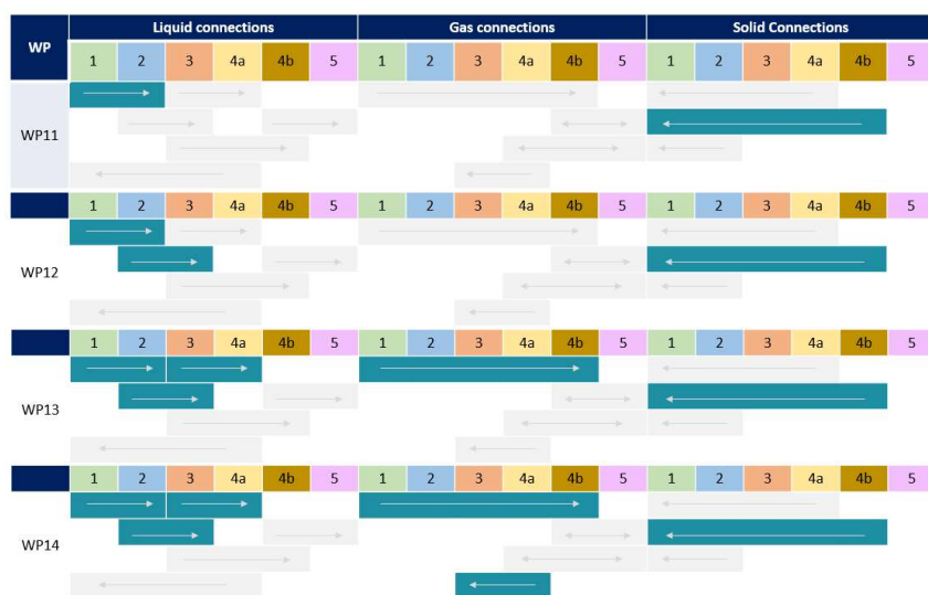
Figure 1-7. Description of WP11 to WP14. Linear liquid loop integration. In this schematic representation, the different air-liquid-solid connections previewed for all compartments are summarized. Interphase's connections that are performed in a specific integration package are highlighted in blue whereas other interphases connections that are included as additional information are highlighted in light grey.
