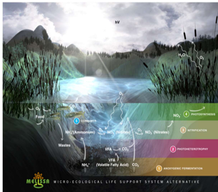
Figure 1-2. Description of the MELiSSA concept. General scheme of a terrestrial ecosystem where the main biological transformations embraced in MELiSSA are highlighted.
