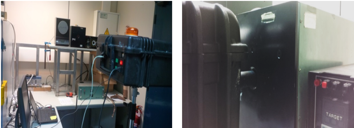
Figure 4.3: Acquisition system under calibration set-up. (left) System on the calibration room close to the blackbody furnace, (right) Close-up.
