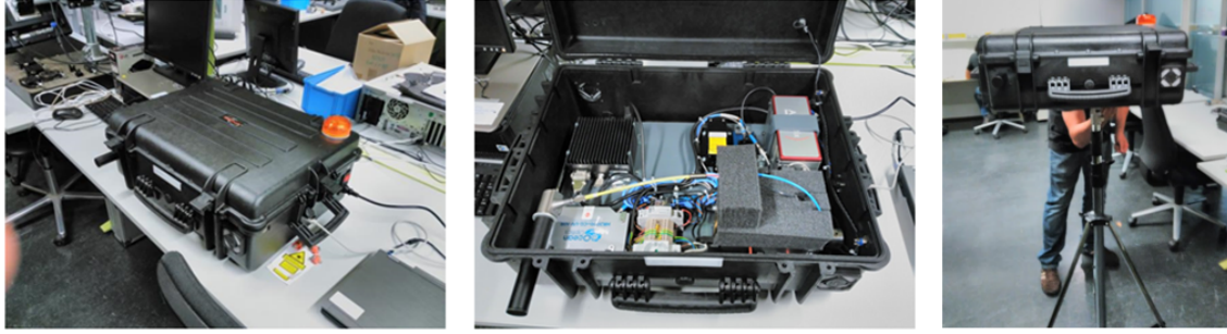
Figure 4.2: Packed prototype. (left) Acquisition case, (middle) Packed opto-mechanical system, (right) Tripod mounting.
