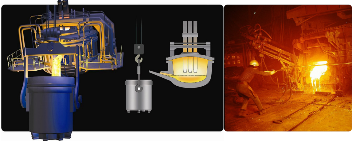
Figure 1.3: Left: Illustration of an Electric Arc Furnace (EAF) during tapping of molten steel into a vessel, and cross-section of a furnace showing the electrodes. Right: a worker manually checks the temperature using a thermocouple attached to a long probe while slag is poured. Image: Deutsche Fotothek (CC BY-SA 3.0 DE).
