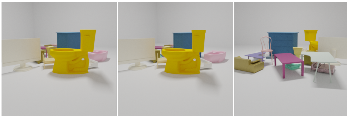
Figure 1.4: Left: object-cluttered 3D scene captured from a reference camera pose. Center: a complementary camera pose featuring a close baseline with respect to the reference ( e.g. those in commercial stereo rigs and typical autonomous driving datasets) results in small disparities and little additional insight over the occluded scene parts. Right: a wide-baseline complementary camera location could potentially provide a substantial information gain over the imaged scene, but the fusion of information from both views and the production of cross-view predictions are far from trivial.
