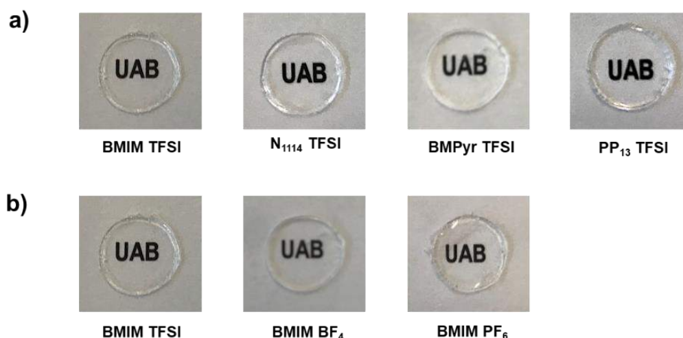
Figure 3.4. Appearance of the different membranes prepared using IL of different chemical nature. a) the IL used have the same anion (TFSI - ) but different cations. b) the effect of changing the anion is observed when BMIM + is used as a common cation.
