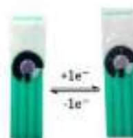
Fig. 7. Performance of ECP-Magenta using state using IG-[BMIM][TFSI] as electrolyte before (left) and after (right) applying 0.4 V.
