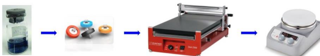
Figure 2.4 Complete fabrication process of PEDOT:PSS thin films. The filtered PEDOT:PSS solution was blade coated and annealed on a hot plate.
