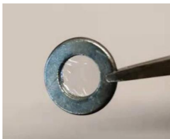
Figure 2.15 Suspended PEDOT thin film on a gasket.
