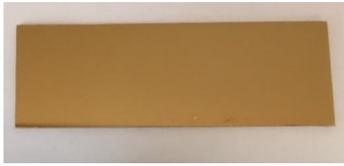
Figure 3.8 A PEDOT:PSS film with a 60 nm gold layer for FDTR measurement.
