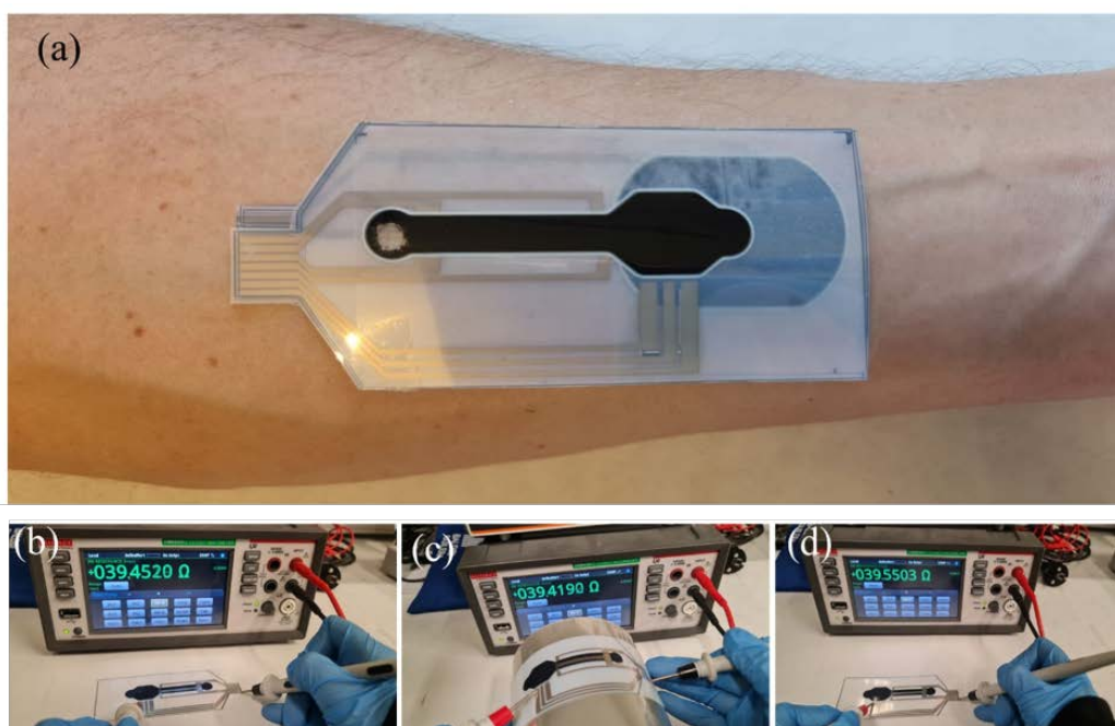
Figure 4.8 (a) The microfluidic device was applied to the distal arm skin. (b) The resistance of connecting the AgNP line without bending. (c) The resistance of connecting AgNP line bent on a cylinder with a diameter of 95 mm. (d) The resistance measurement of the connecting path on the flat substrate after bending.
