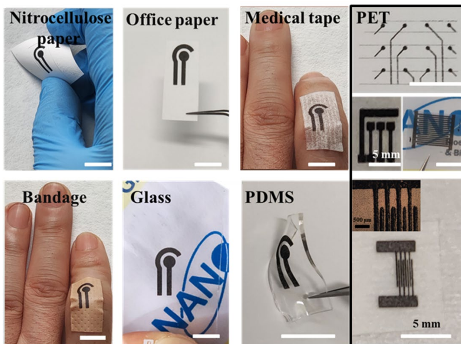
Figure 3.11 T-LRGO on various substrates. The inset picture shows an interdigitated LRGO pattern before transferring. The scale bar is 1 cm unless labelled otherwise.
