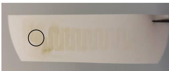
Fig. 5.13 Real image of the damaged gas diffusion membrane. Donor side inlet indicated by a black circle.
