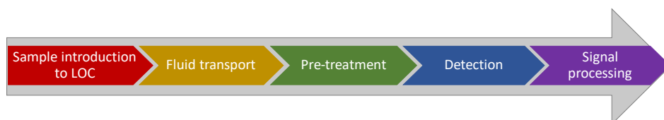
Fig. 1.4 Basic unitary operations for a given analytical process integrated in a \mu TAS.
