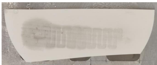
Fig. 4.28 Real image of the PVDF gas diffusion membrane after direct contact with a blood sample.
