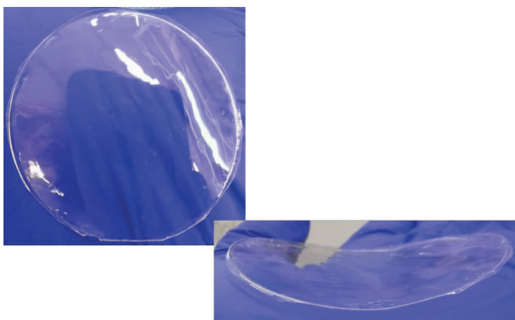
Figure 7.44. Visual inspection of the PVA substrate following immersion in CB
