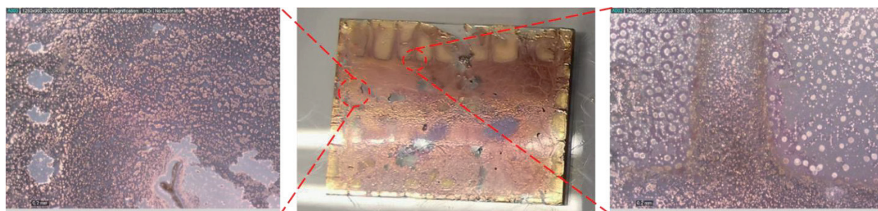
Figure 7.5. Au film development on silk substrate at 31 days (+83 days vacuum sealed)
