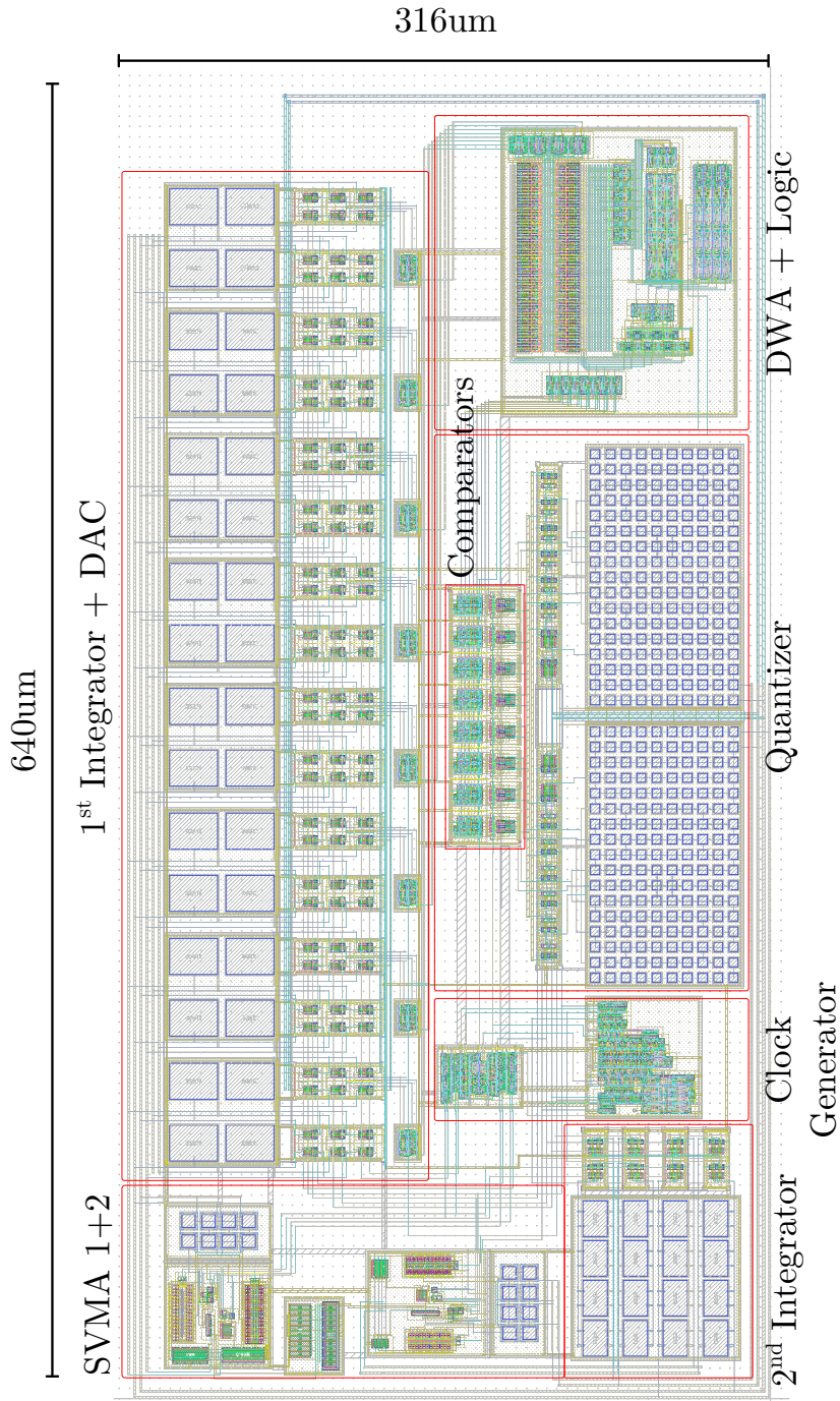
Figure 5.2 | Layout design of the Multi-bit \Delta\Sigma in 180 nm CMOS technology. Total design area is 0.202 mm 2
