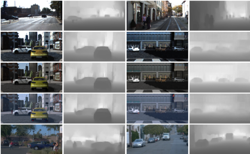
Figure 2.3: RGB images with their estimated depth. From top to bottom rows: samples from \mathcal{K} , \mathcal{V}_{g_{\mathcal{K}}} , \mathcal{V} , \mathcal{V}_{g_{\mathcal{W}}} , \mathcal{W} . The samples of \mathcal{V}_{g_{\mathcal{K}}} and \mathcal{V}_{g_{\mathcal{W}}} correspond to transforming the samples of \mathcal{V} to \mathcal{K} and \mathcal{W} domains, respectively. The monocular depth estimation model [130] was trained on the \mathcal{K} domain.
