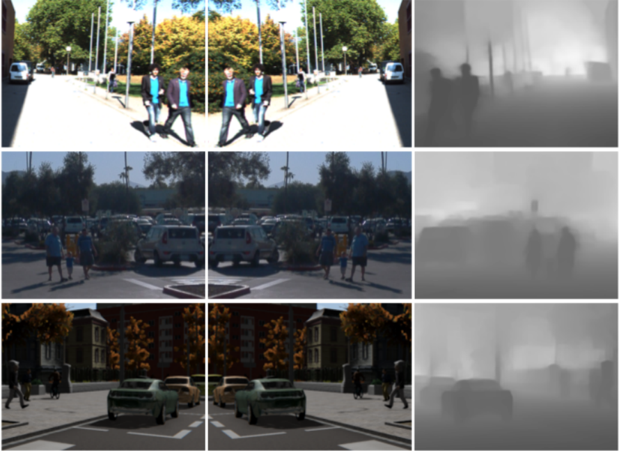
Figure 2.1: From top to bottom: samples from KITTI ( \mathcal{K} ), Waymo ( \mathcal{W} ), and Virtual-world ( \mathcal{V} ) datasets. Middle column: cropped patch from an original image. Left column: horizontal mirror of the original patch. Right column: monocular depth estimation [130] from the original patch. Left-middle columns are the views used for co-training in [110]. Right-middle columns are the views also used in this chapter.
