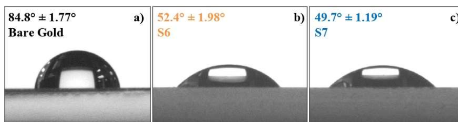
Figure S8: Contact angle measurements of a) bare gold, b) S6 and c) S7. A drop of 3 \mu L of Milli-Q water was used for these experiments.
