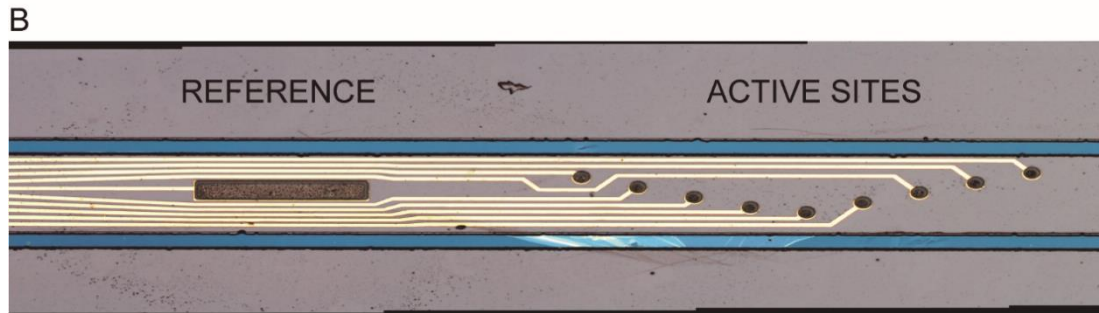
B) Image of a section of a fabricated probe with 9 graphene microelectrodes (black dots) plus a reference (black rectangle). For more details see Viana et al., 2022.
