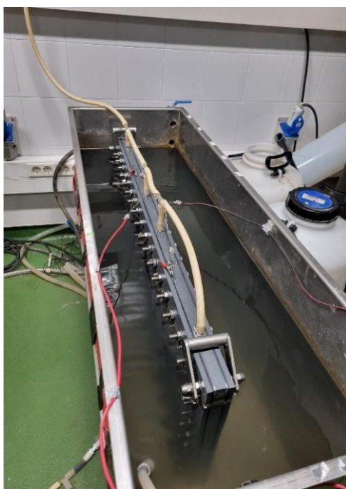
Figure 6.2. Experimental set-up during the performance evaluation of a cassette with synthetic wastewater in the L-MEC.
