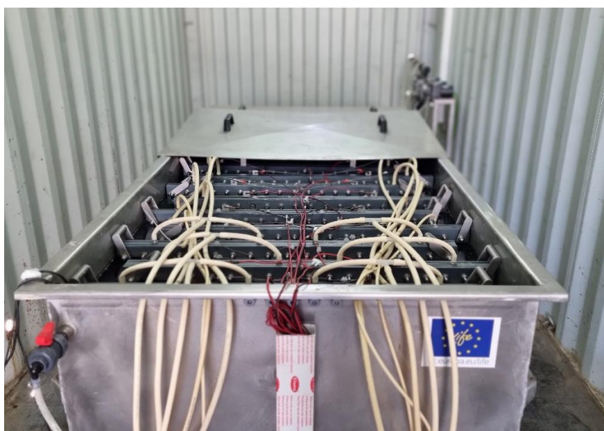
Figure 6.4. Experimental set-up during the performance evaluation of the M-MEC with ten cassettes with urban wastewater.
