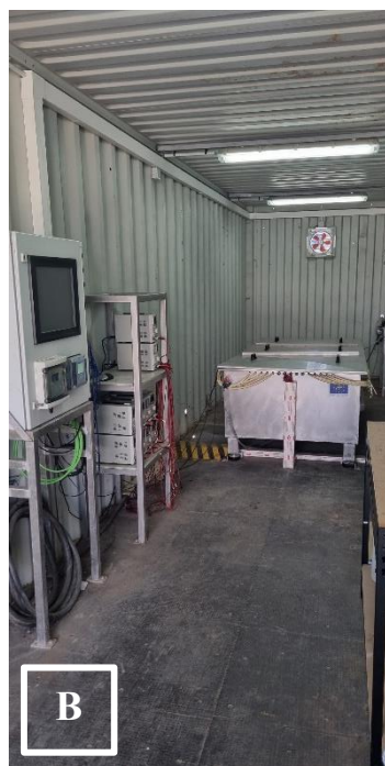
Figure 6.11. A) Shipping container located next to the primary settlers; B) Monitoring system and power sources; C) M-MEC; and D) Different cassette-type cells placed inside the reactor.
