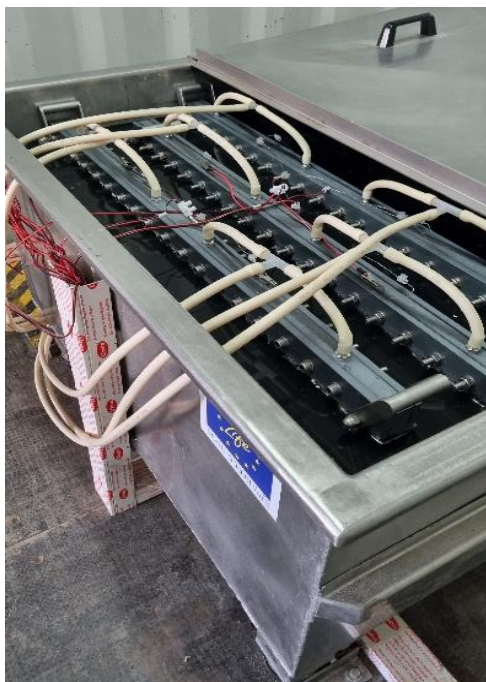
Figure 6.3. Experimental set-up during the performance evaluation of three cassettes with urban wastewater in the M-MEC.
