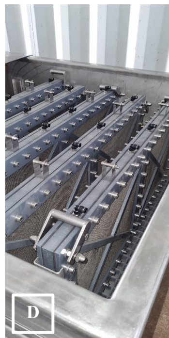
Figure 6.11. A) Shipping container located next to the primary settlers; B) Monitoring system and power sources; C) M-MEC; and D) Different cassette-type cells placed inside the reactor.
