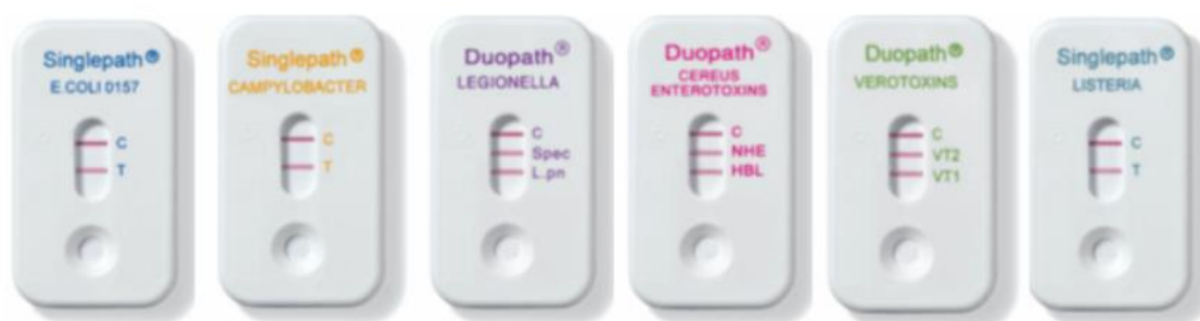
Figure 1.12. Commercial lateral flow strip Singlepath® and Duopath® for the detection of different bacteria from Merck (Germany).
