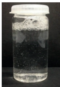
Figure 2.20: Temporal aggregate formation when mixing CTAB and rhEGF in the aqueous phase to prepare rhEGF-DELOS nanovesicles, rhEGF:CTAB ratio (mmol:mol) = 0.6.
