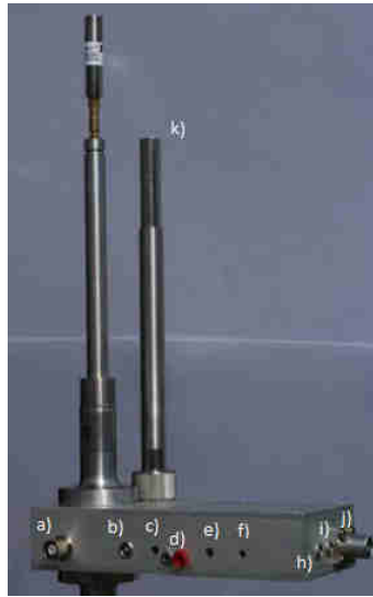
Figure 4.35: A view of the proportional tube, special Al tube (k) and the metallic box where the associated electronics to the proportional counter is found. High voltage is set through input a. Low voltage is set through input j. Analog pulses are sent through output i. Digital pulses are sent through output h. Pulse tests can be done through output b. Pulse height discriminator is set through entrance c. Voltage of the applied discrimination is measured in d. Gain can be modified e. The configuration of the previous parameters can deleted through entrance f.
