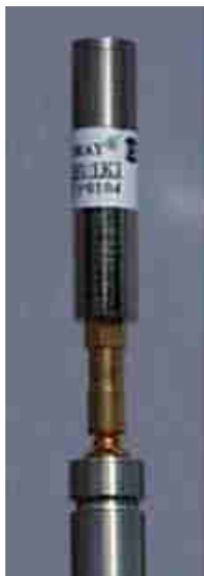
Figure 4.33: UAB proportional counter. From Bakali [2001].
