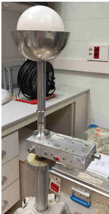
Figure 4.43: Situation in which Cd shell is used. Only half of the Cd shell is shown to make the sphere visible. The pertinent moderating sphere will be closed inside the shell.
