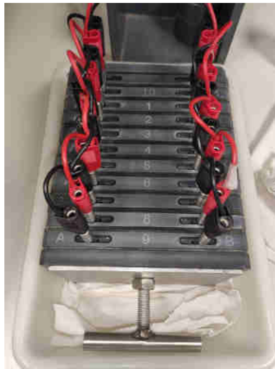
Figure 4.29: In the tiny holes the 0.25 M KOH and 6 M KOH dissolutions are properly introduced so each PADC layer in its irradiated face will meet with the 6 M KOH dissolution. Gray metallic electrodes are in contact with the dissolutions. Black and red cables transport the electric potentials so that each PADC will be under a potential difference.
