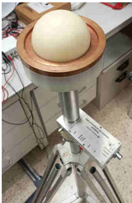
Figure 4.44: Situation in which the 1 " thick Cu shell will be placed between the 4 " moderating sphere and 0.5 " thick polyethylene shell.
