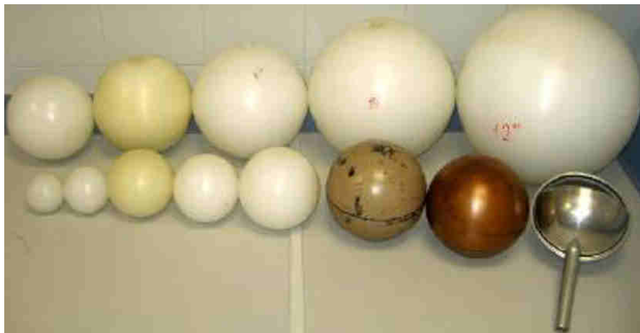
Figure 4.36: Polyethylene spheres, Pb mounted shell, Cu mounted shell and Cd shell.
