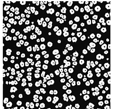
Figure B.6: R = 1461 \text{ tracks cm}^{-2} . H = 10 \text{ mSv} . CR-39 labelled as 1345. The image has dimensions 4 \text{ mm} \times 4 \text{ mm} .
