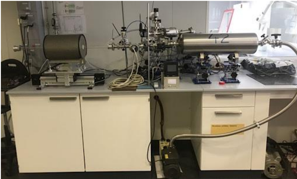
Figure 2.5. P-route oven setup for the preparation of YBCO samples through the TLAG-CSD method.
