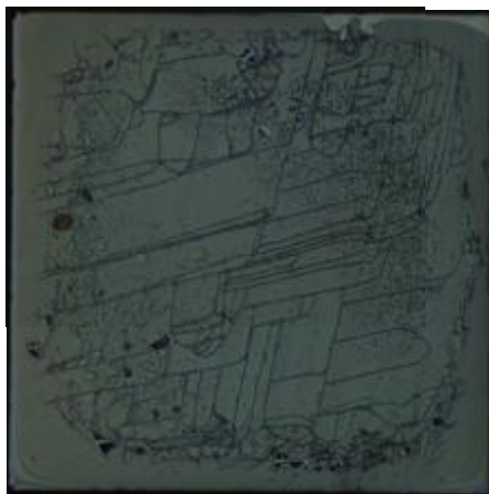
Figure 3.15. 15/1/3 °C/min pyrolysis profile (or B). The precursor solution was FF-B2 with 10%vol. varnish using a deposition matrix of (125x15µm).
