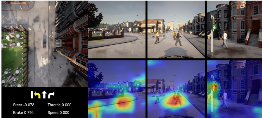
Figure 4.7: Activation maps of CIL++ at an intersection in Town 2. Three image areas from different views are highly activated: the traffic light in the right image, the crossing pedestrians in the central one, and the lane shoulder in the left one. Causality between observation and action is shown as strong braking (0.794) due to the pedestrians, even though the traffic light is green and the turn-left command.
