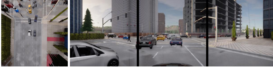
Figure 4.5: An example of traffic deadlocks in Town 5 that could lead to a timeout in route completion.
