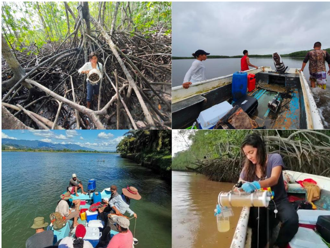
Figure 4. Sampling campaigns carried out in the Térraba-Sierpe Wetland. Top-left: Mollusc extraction in the mangrove forest. Top-right: Access to the sampling site during low tide. Bottom-left: Water characteristics measurement. Bottom-right: Water sampling with Niskin water sampler.
