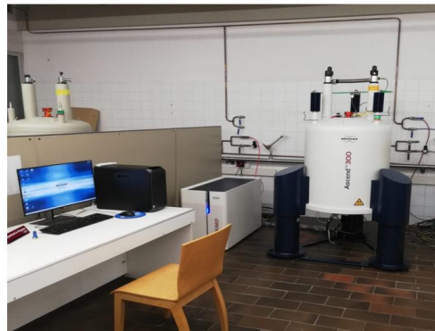
Figure 3.1.1 (A) 7T Bruker Biospec 70/30 USR scanner and (B) High resolution 300MHz AVANCE NEO spectrometer at the SeRMN UAB.
