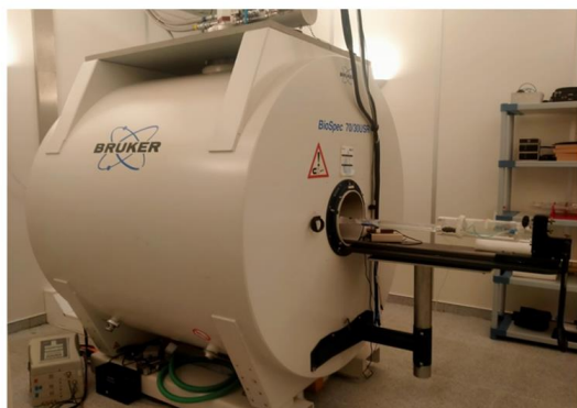
Figure 3.1.1 (A) 7T Bruker Biospec 70/30 USR scanner and (B) High resolution 300MHz AVANCE NEO spectrometer at the SeRMN UAB.
