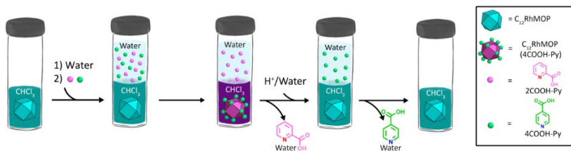
Scheme 4.4 Schematic representation of the selective extraction of 4-COOHPy to the CHCl_3 phase and its subsequent recovery in the aqueous phase.
