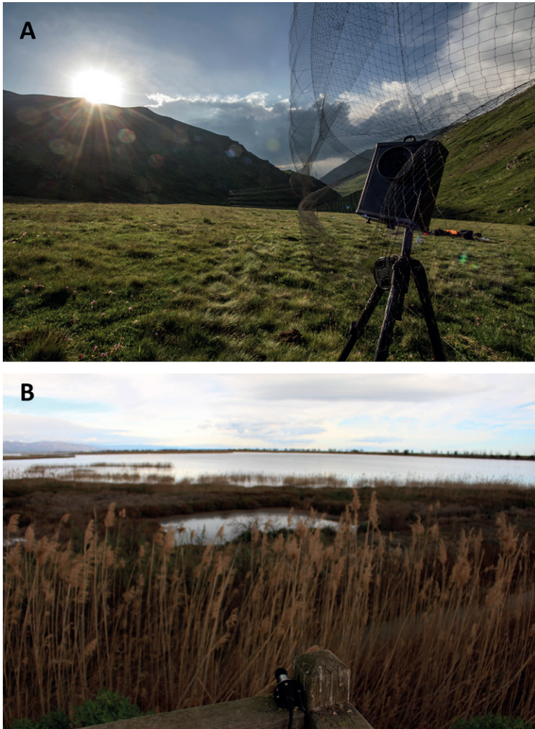
Figure 1.8: Two different ultrasonic devices used to monitor bat populations. A) Batlure placed near mist nets to improve the capture ratio in alpine meadows. B) Ultrasonic bat detectors placed in a lagoon to record the bat activity in open wide areas. Upper photo courtesy of Adrià López-Baucells; bottom photo courtesy of Maria Mas.
