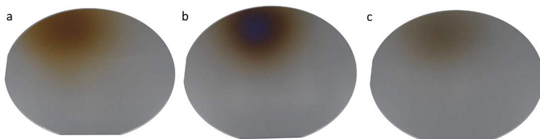
Figure 2-3. Deposition of ceramic perovskites on Si (100) wafers: LSM, LSF, and LSC, respectively (a-c).
