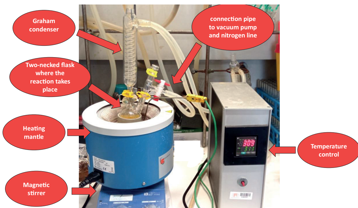
Figure A42: Assembly for the second step of \text{LiYF}_4:\text{Yb}^{3+},\text{Tm}^{3+} synthesis
