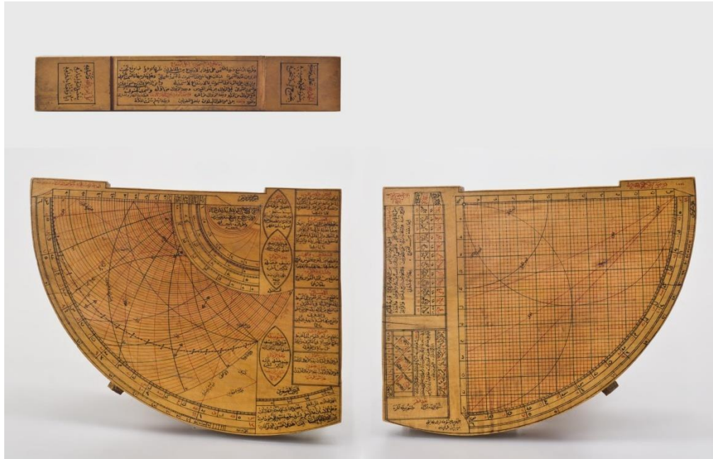
Figure 35. Astrolabe-quadrant from Ottoman empire, solid walnut, inscribed in red and black ink under a yellowish varnish; brass socket for the plumb-line; the lead weight for the plumb-line is housed in the instrument. 16.8 x 12.8 x 3 cm; radius of quadrant 12.5 cm. One side of the instrument carries a Prophatius astrolabe-quadrant for latitude 41^\circ , with an unequal hour diagram (horary quadrant) above. The other side is a sine-cosine quadrant with arcs of sine and versed sine. There are brief instructions in Turkish and Arabic on the sides and edges. The maker's name appear on each side, with slight variations in some details of the signature. The nisbah of the maker, al-Ufi, indicates that he was from Of, a small town on the Black Sea. Estimated 16th century.
