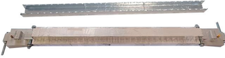
Figure 4.21 Full view of the waveguide cavity and the unidirectional LWA arrangement.
