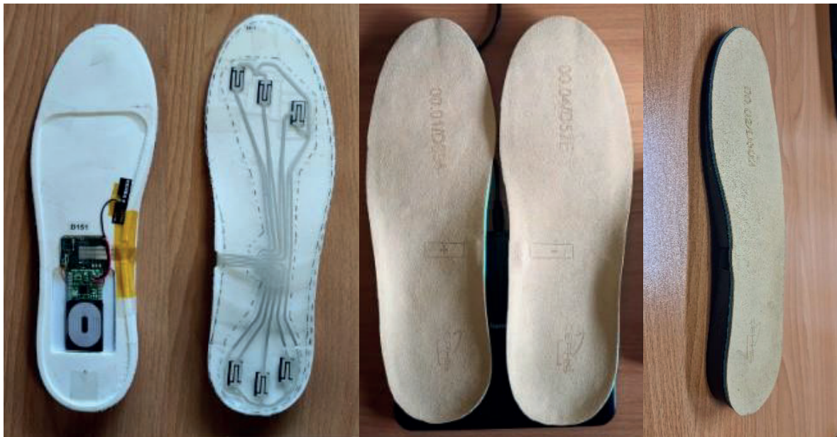
Figure 18: Developed insoles. View of electronic and sensors, and finished product.
