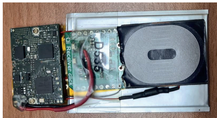
Figure 7: Integration of PCB, Qi charging module and Battery.
