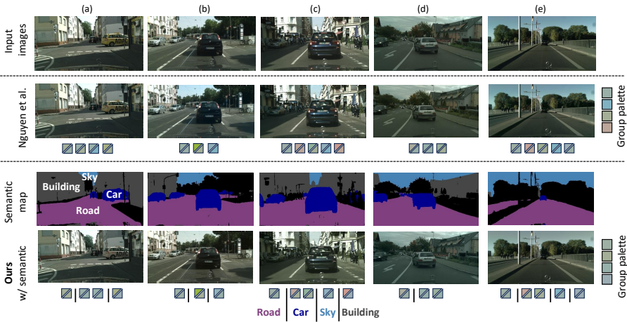
Figure 3.8: Results of adding the semantics-guided module. From top to bottom: Input images from Cityscapes [32], the result of Nguyen et al. , the input semantic maps predicted by the Slim-DeepLabv3 model in Chapter 2, and our recoloring results. There is noticeable noise in the “road” region of the semantic segmentation prediction. However, our method is still able to achieve color-consistent recoloring results under the guidance of such noisy semantic maps. Particularly, in the regions of the “car” in column (a) and (c), our method obtains more consistent colors compared to the results without semantic guidance.
