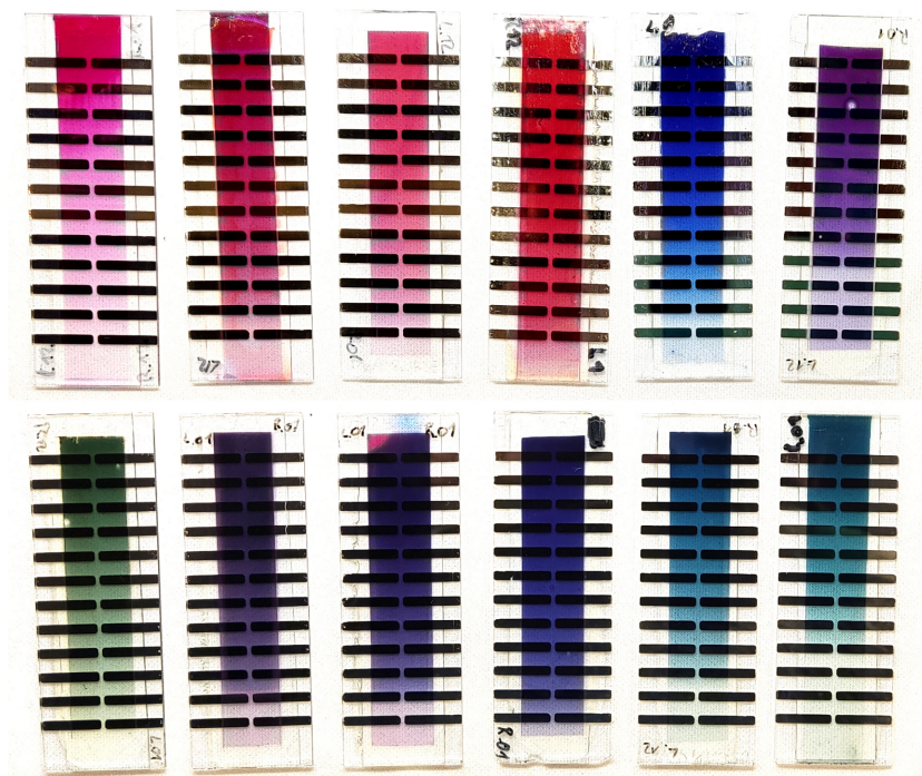
Figure 2.7: Compilation of OPV samples fabricated during the thesis. The active layer materials of the top row (from left to right) are: D18MI-FF-PMI; PTQ10:O-IDTBR; P3HT:PC 60 BM; P3HT:O-IDFBR; PM6:IO-4Cl; PTQ10:PC 60 BM. The active layer materials of the bottom row (from left to right) are: PTB7-Th:PC 60 BM; P3HT:O-IDTBR; P3HT:EH-IDTBR; PTQ10:Y6; PTB7-Th:Y6; PTB7-Th:COTIC-4F. The IUPAC name and chemical structures of some of the materials are not included in the active layer materials since they are not included in any results of the thesis. This figure is only for the sake of art.
